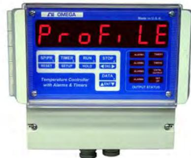
Upon entering the process profile mode, display will first read **Strt SP** very briefly and then the current value of Starting setpoint. Use '^ENTv' and '<DIG >' keys to enter a desired value. The '^ENTv' key increments and decrements the FLASHING digit, where as the '<DIG>' key selects the digit to increment or decrement. Next, press the 'SETUP' key to go on to the next function.
