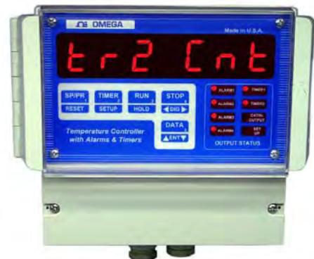
To display Timer #2 value, push TIMER key three times. First two pushes display elapsed time and timer 1 value respectively, while the third push brings up timer 2 value on the display. This is, however, preceded by the message 'tr2 Cnt' (for Timer 2 Count).
