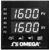
Experienced users, already familiar with the Series CN8200, and using the controller with PID outputs, may follow these condensed instructions to autotune the controller and get started quickly once the instrument is properly mounted and wired, and the Security Level is set to **CONF**. Once setup is complete, we recommend changing the Security Level back to the most restrictive level suitable for your application.
