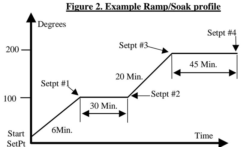
From '**VERIFY**' display press  $\wedge$ v key until '**PrOFILE**' (Enter Ramp/Soak) is displayed.
