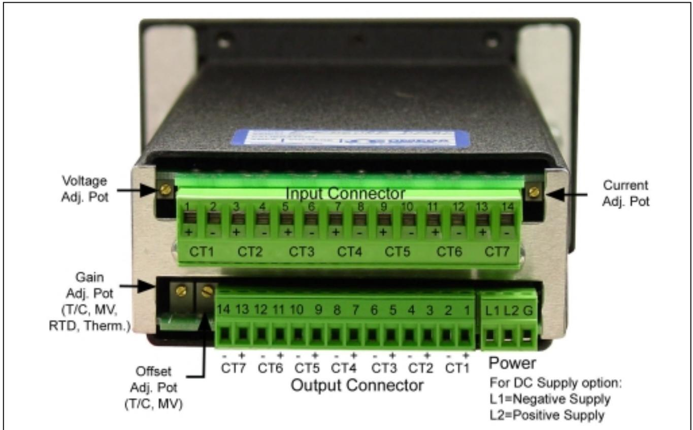
**INPUT/OUTPUT CONNECTORS PIN ASSIGNMENTS**
