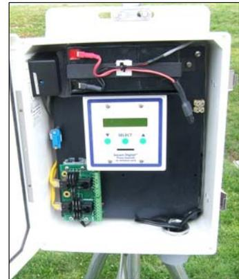
WMS-25-NEMA-DL Data Logger in NEMA Enclosure
