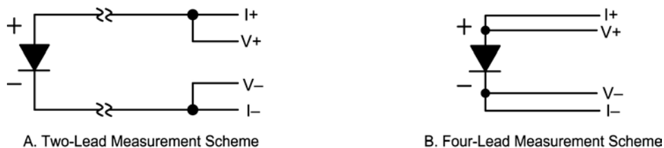
Figure 1. Two-Lead Versus Four-Lead Measurements
