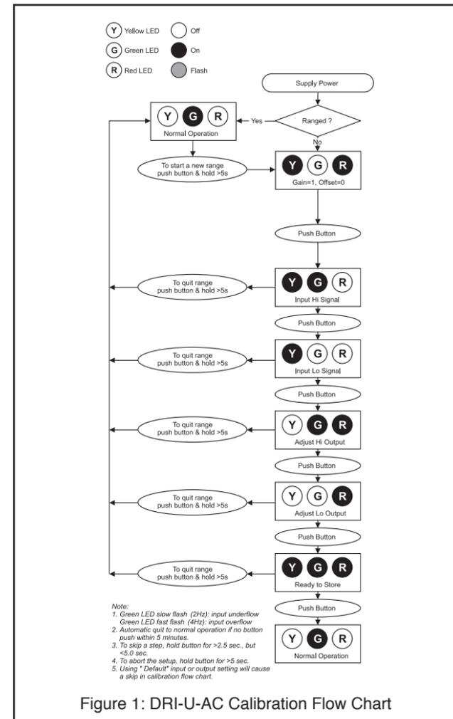
Figure 1: DRI-U-AC Calibration Flow Chart
