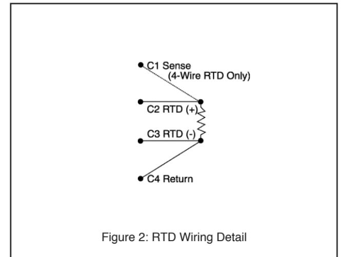
Figure 2: RTD Wiring Detail
