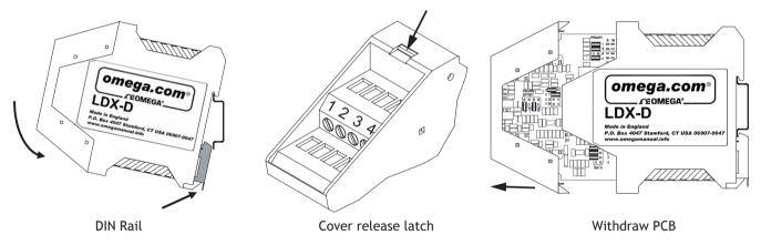
To access internal links, the front cover and PCB must be withdrawn from the housing. Use a screwdriver or similar tool to depress the top latch. The cover will spring forward. Repeat with the bottom latch, then gently pull the PCB out.
