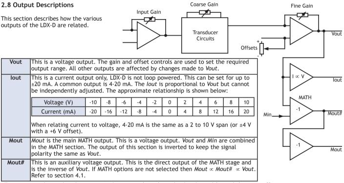
All outputs may be used at the same time but cannot be independently adjusted for scalefactor or offset.
