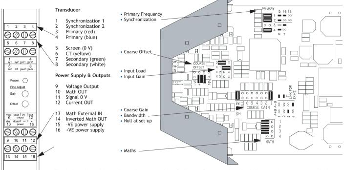
Terminals 5, 11, and 15 are internally connected but, for best performance, they should be treated as separate terminals. Note: If the output polarity is incorrect, reverse the transducer secondary connections
