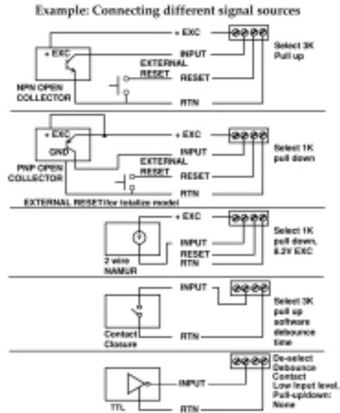
3. Connect the signal input to screw terminal, and ensure that the screws are tight
