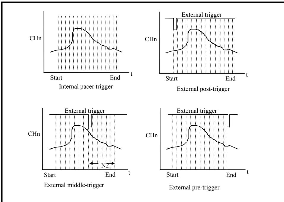
Figure. 1-2. Trigger modes of OME-PCI-1202/1602/1800/1802.
