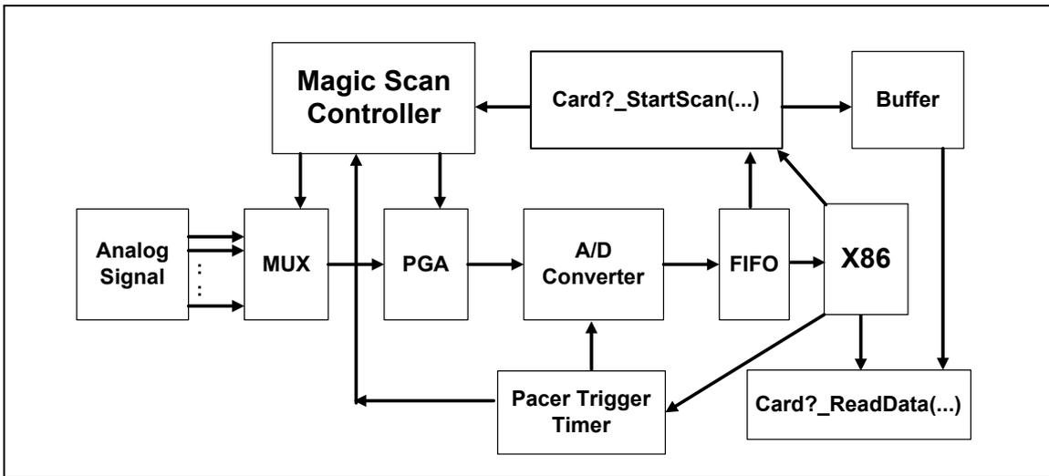
Figure 6-1: The block diagram of the continuous capture.
