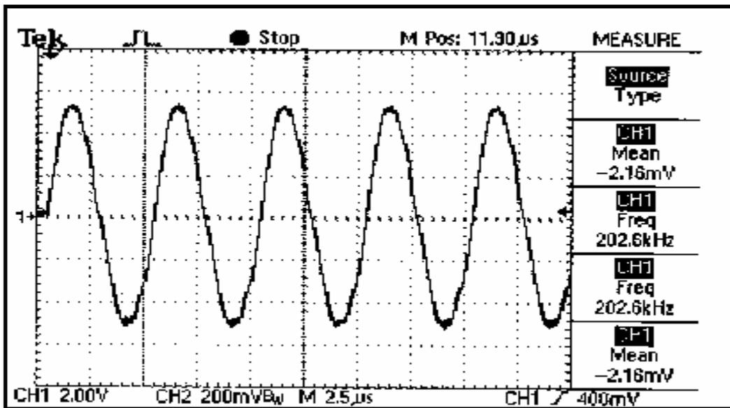
Figure 5-4: The M\_Function\_1 used to create a 200K, +/-5V sine wave.
