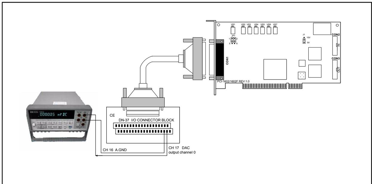
Figure 7-2. D/A Calibration
