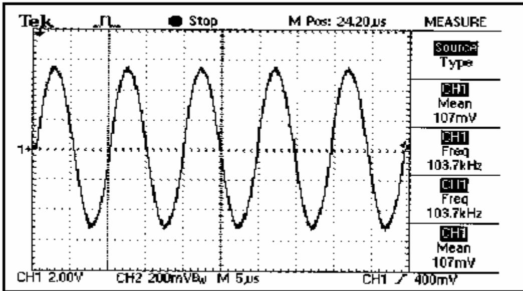
Figure 5-3: The M\_Function\_1 used to create a 100K, +/- 5V sine wave.
