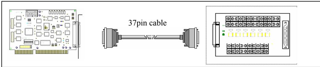
**A.5: Connection to OME-PCI-1x02 and multiple OME-DB-889D (16 channels differential)**
