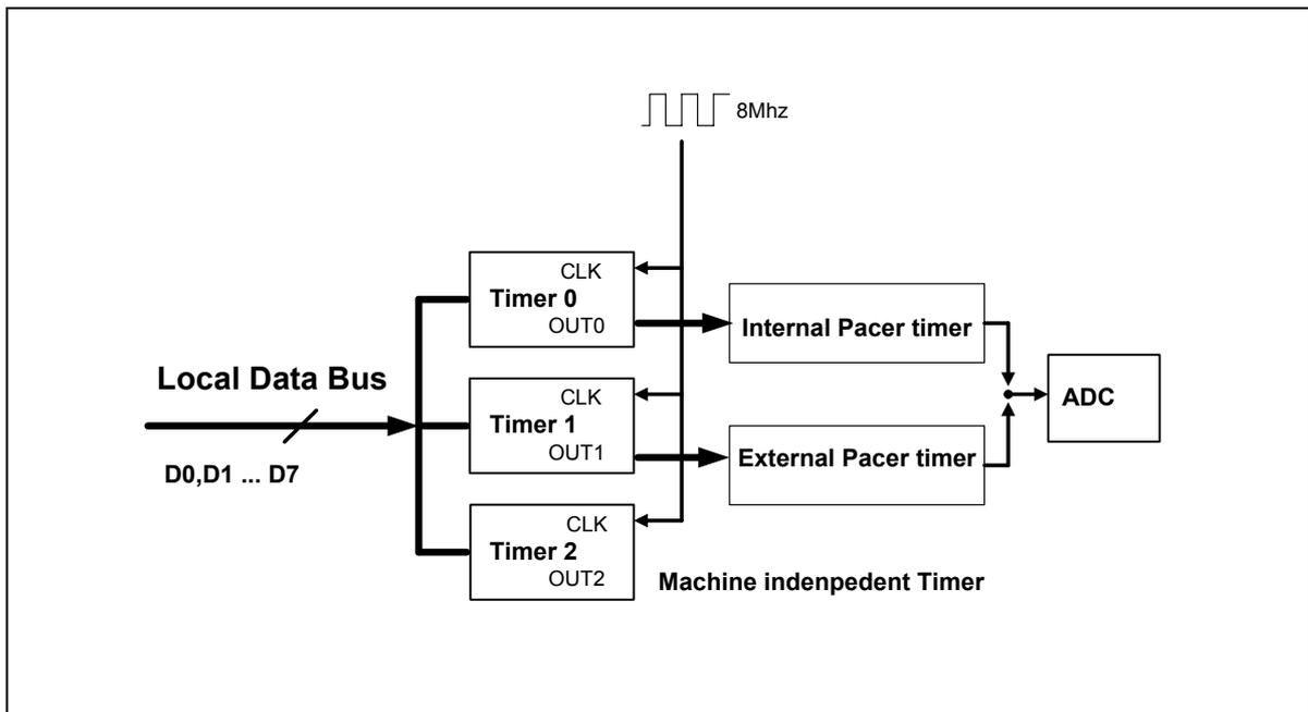
Figure 3-1: The block diagram of OME-PCI-1202/1602/1800/1802 8254 timer.
