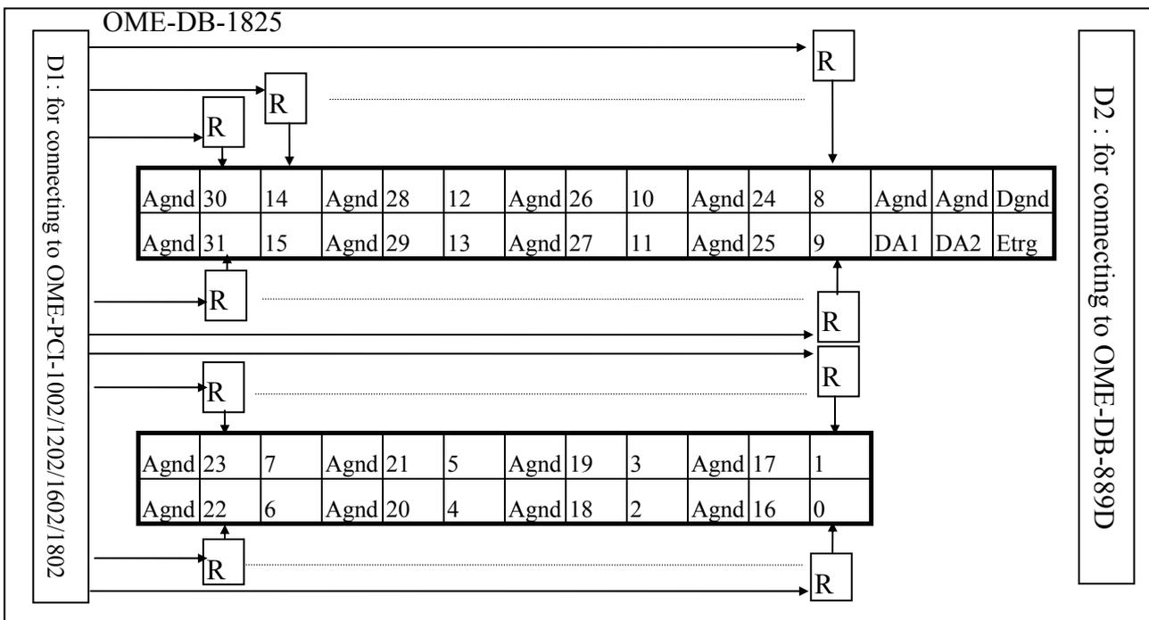
Pin assignment of D1 same as **CON3** of OME-PCI-1002/1202/1602/1802
