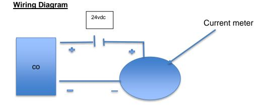
Scaled 4-20mA loop powered = 0-50ppm
