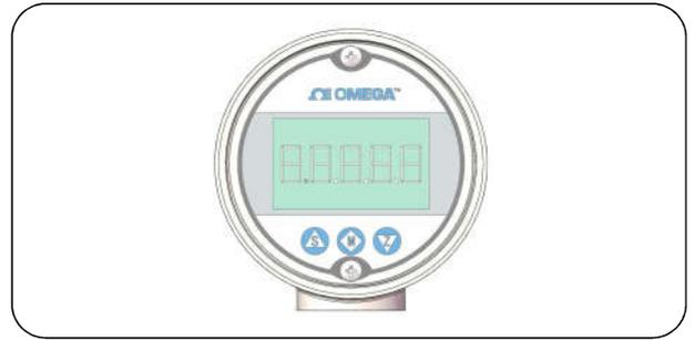
Adjustments to operating parameters can be done by removing the protective cover. When commissioning is complete, replace cover, taking care not to cross thread, and tighten snugly by hand.
