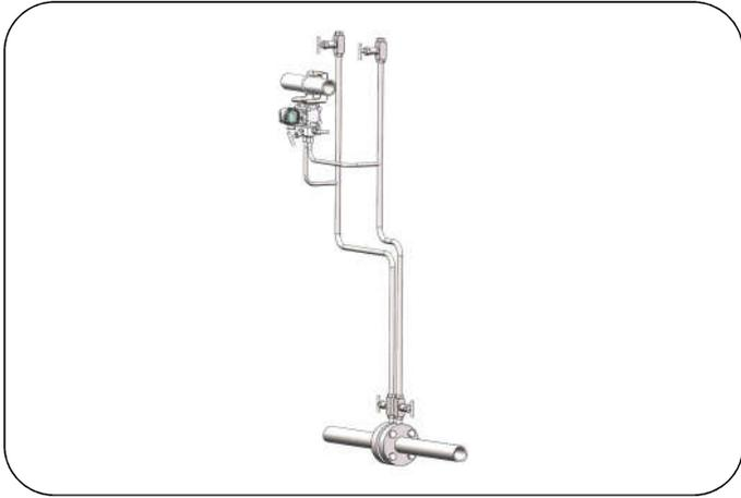
The pressure tube should be tilted up 45°, the installation location should be lower than the process pipeline. Isolation tank and multiple shut-off valves should be used. Open the drain/vent valve periodically to clear the residual gas and liquid in the guiding pressure tube to ensure accuracy.
