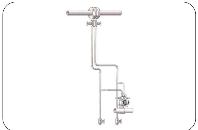
The pressure tube should be tilted down 45°, the installation location should be lower than the process pipeline. Isolation tank and multiple shut-off valves should be used. Open the drain/vent valve periodically to clear the residual gas and liquid in the guiding pressure tube to ensure accuracy.
