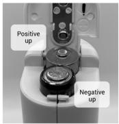
Note: Positive side of the battery has a "+" mark and negative side has a "-" mark on the battery label.
