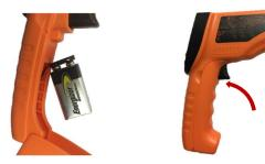
Attach a 9V battery (provided) to the black connector inside. The battery should snap into place. Swing the front of the handle back upwards to close the unit.
