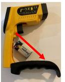
Insert the 9V battery into the battery holder.
