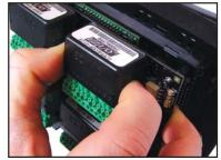
Caution: Do not use AC output module in the bottom left slot due to height of the battery. Analog IN/OUT module can be used only on the first 4 slots. Other analog modules or High Speed counter module can be used only in the first ten slots.
