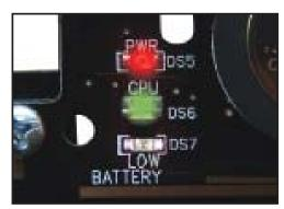
Red Power LED indicates that the PLC has power. Green CPU LED indicates that the CPU is executing a valid program. Red Low Battery LED will momentarily turn on at Power ON and then stay off if the battery is good. If the battery is low, this LED will turn on.
