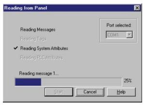
**Ensure that the EZSeries Text** Panel(s) is in SETUP Mode **BEFORE** attempting to Read or Verify Project. If it is a Multi-Panel Project, ensure that the EZ Multiplexer is in PROGRAM Mode (Mode
