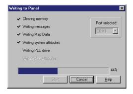
Ensure that the EZSeries Text Panel(s) is in SETUP Mode BEFORE attempting to Write Project. If it is a Multi-Panel Project, ensure that the EZ
