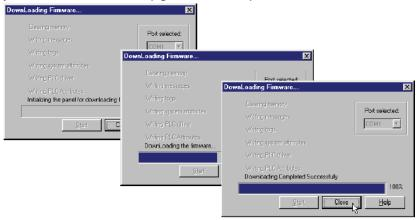
When you initialize the **Upgrade Firmware** process, the EZSeries Text Panel Message display will read **SELF TESTING**. When the download begins, the display will read LOADING EXEC. When the download is complete, the panel will enter the Run Mode.
