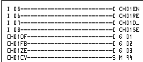
Figure 75: EZ800 Control Relay circuit diagram with high-speed counter
