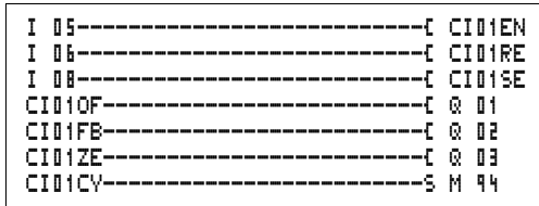
Figure 77: EZ800 Control Relay circuit diagram with high-speed incremental encoder counter
