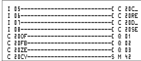
Figure 71: EZ800 Control Relay circuit diagram with counter relay
