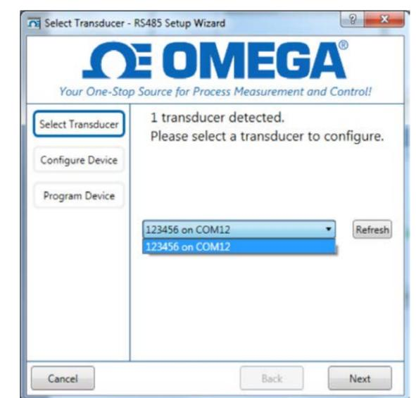
Figure 4: Select Transducer Screen
