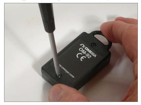
Then remove the circuit board from the box (use soft tool or fingernail to remove)
