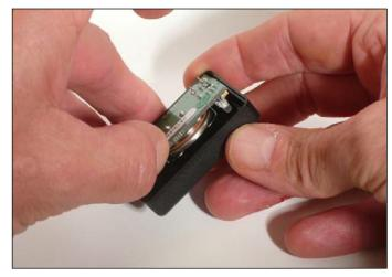
Insert a new battery as shown being careful not to touch and exposed electronics in the process.
