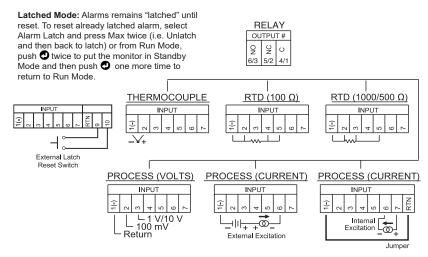
Connect the main power connections as shown in the figure below.
