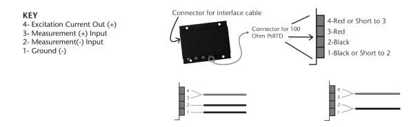
For 3-wire RTD probes, short inputs 3 and 4 together, then connect the lead wires to input 1, 2 and 3. For 2-wire RTD probes, short inputs 3 and 4 together and inputs 1 and 2 together, then connect the RTD lead wires to inputs 2 and 3.
