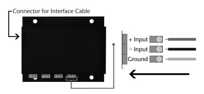
Warning: Note the polarity instructions. Do not attach wires to the wrong terminals.
