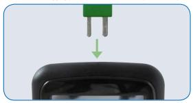
The device is configured to a K type probe. If you wish to use a J, N or T type probe select the Settings button and choose the correct probe type.
