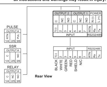
Refer to Operator's Manual for important Input Probe Note Shield wiring notes
