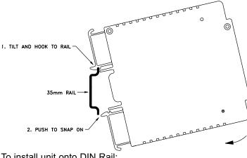
To install unit onto DIN Rail:
