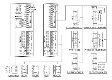
Connect the main power connections as shown in the figure below.
