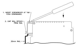
To remove unit from DIN Rail:
