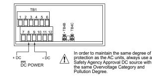
**DC Powered Unit Connections**
