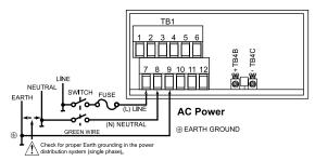
**AC Powered Unit Connections**
