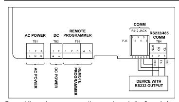
Connect the main power connections as shown in the figure below.
