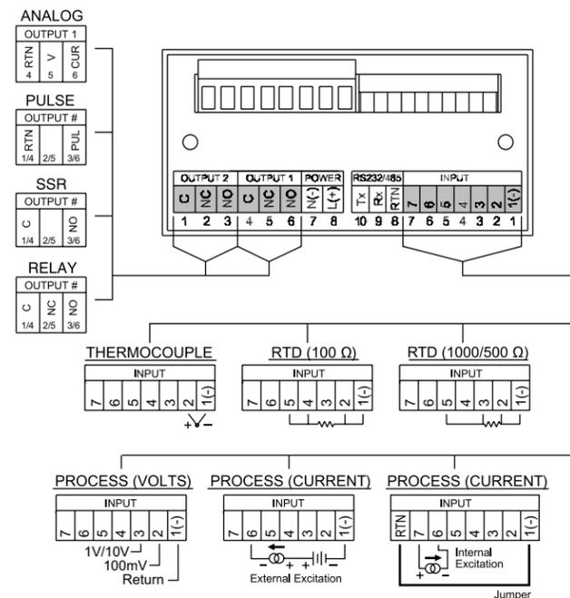
Connect the main power connections as shown in the figure below.
