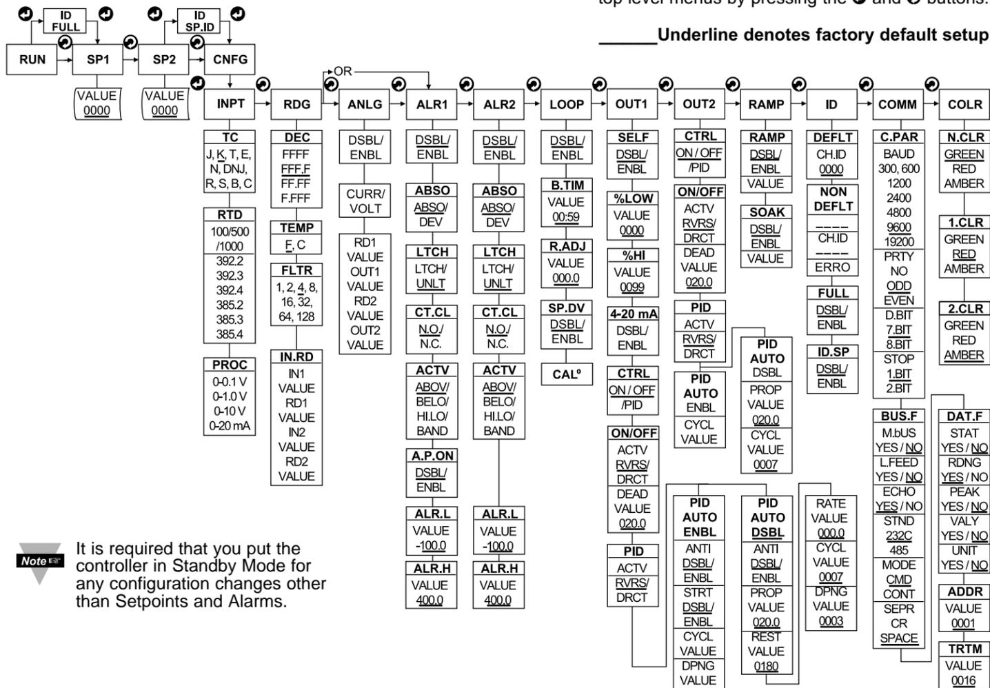
Below is a flowchart showing how to navigate through all top level menus by pressing the **↶** and **↷** buttons.
