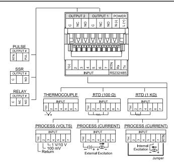
Connect the main power connections as shown in the figure below.
