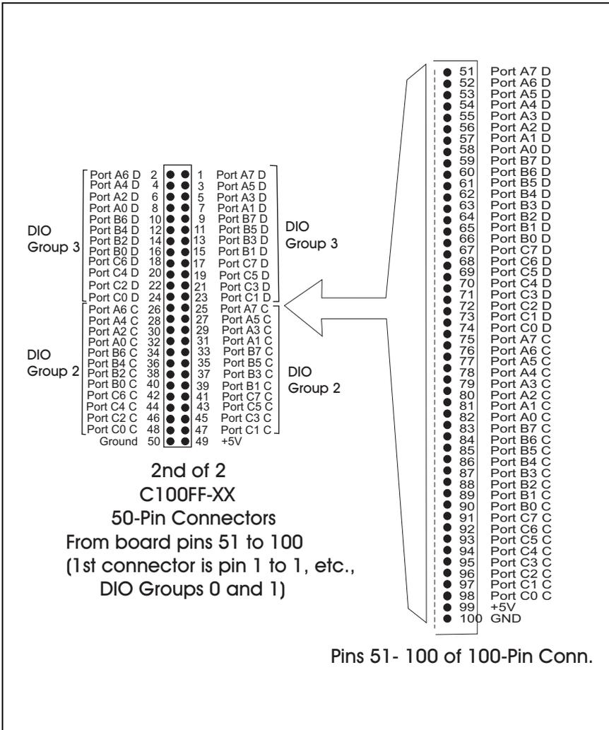
Figure 3-3. Pin Translation - Pins 51 to 100 DI/O Signals
