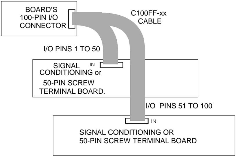
Figure 3-2. Cable C100FF-xx Configuration
