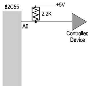
Figure 7-1. Pull-up Resistor
