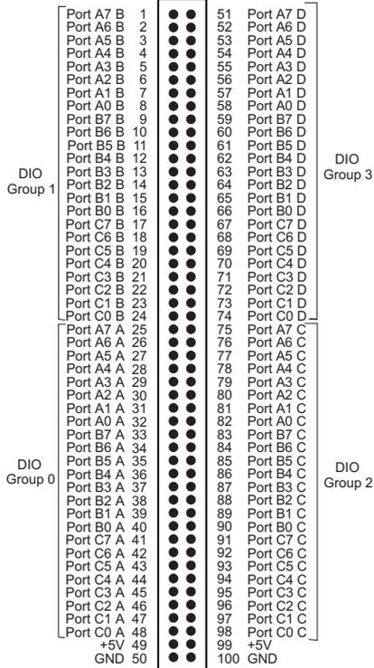
Figure 3-1. PCI-DIO96 100-Pin Connector Pin Out
