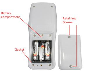
Figure 1: Battery Installation
