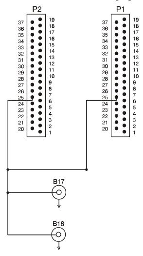
The BNC-16DI incorporates 16 front panel mounted BNC's allowing connection of up to 8 differential analog inputs to the CIO-DAS and PCI family of data acquisition boards. The BNC-16DI can accommodate boards with either 37 or 50 pin I/O connectors; with connector P2 used to interface to data acquisition boards utilizing a 37 pin, D type I/O connector, while connectors P3, P4 and P5 are used to interface to data acquisition boards utilizing a 100 pin I/O connector.
