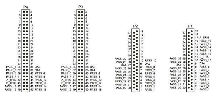
P1 Connector Map for BNC-16SE and BNC-16DI
