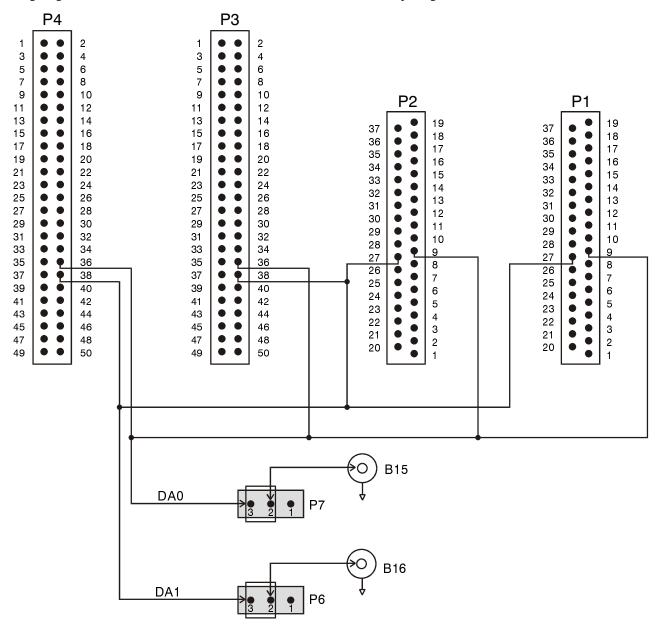
Connector P1 provides the user with a variety of I/O signals, <u>not</u> including the 16 analog input signals from B1-B16. The following diagram illustrates the connection scheme used to route these signals among connectors P2, P3 and P4 to connector P1. These signals are labeled "PASS" signals (except for the trigger and D/A options as shown) and the user should consult their DAS manual's I/O connector pin assignment section to verify the actual signals available at the P1 connector.
