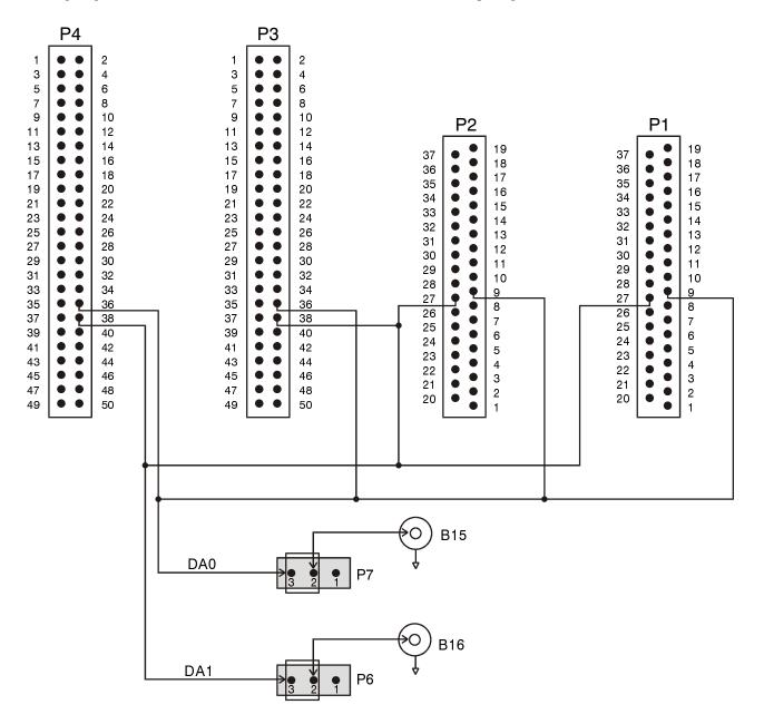
The BNC-16SE incorporates 16 front panel mounted BNC's allowing connection of up to 16 single-ended analog inputs to the CIO-DAS and PCI family of data acquisition boards. The BNC-16SE can accommodate boards with either 37 or 50 pin I/O connectors; with connector P2 used to interface to data acquisition boards utilizing a 37 pin D type I/O connector, while connectors P3, P4 and P5 are used to interface to data acquisition boards utilizing a 100 pin I/O connector.
