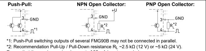
Ensure that the maximum signal current of 25 mA is not exceeded.
