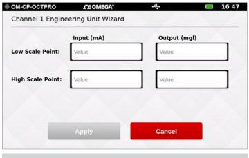
Enter the low and high scale point inputs and outputs and click Apply.
