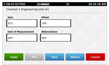
The gain and offset are automatically set. Click **Save** to save the engineering units to the channel and click Apply to apply the changes to current logging session.
