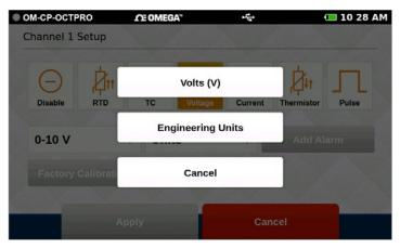
Engineering Units: This will be an option to set up if the user selects the Voltage, Current or Pulse sensor (see details below and on page 9-10).
