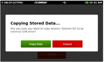
**Note:** Data can be saved to external memory as .csv and/or .mtb file format (user selectable in System/File Format). Saving as .mtb file format will allow data to be imported into Omega 4 Data Logger Software (version 4.2.13.0 or greater).
