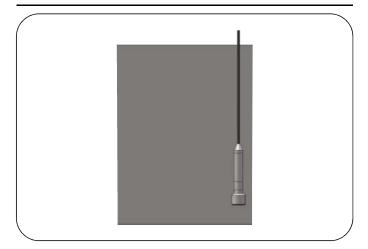
In cases were a protective tube is unable to be used, a counterweight can be used to stabilize a transmitter in fast flowing areas.
