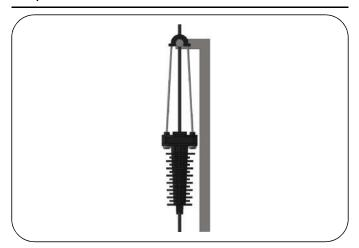
Clamps can be used to fix and support the entire product for direct cable connection level transmitter. Cable outlet should be of sufficient length to be directly connected to the control room, or adapter junction box, avoid bare connections in the field environment.
