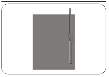
For products with more than 50 meters cable, the wire rope and cable bundled multi-point should be used to strengthen the level transmitter support.
