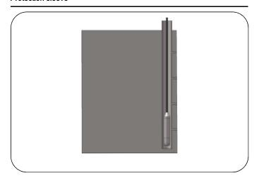
Submersible Level Transmitter should be suspended inside the protective sleeve to avoid the impact on the level transmitter from fast flowing medium.
