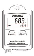
**Turn Off the Logger -** Push the "LOG/STD" Button for 5 Secs then LCD display is off.
