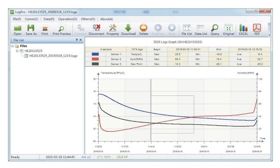
Tips: Press and hold the left mouse button to drag a box, when the left mouse button is released, the graph will be redraw with the data in the selected rectangle area. Click right button, then the graph will be redrawing with all the data in the logs file.
