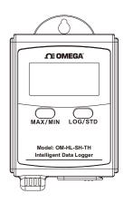
**LOG Full -** The device won't record data while the memory is full, that you have to download the data and delete it by Logpro software, then device can record again.
