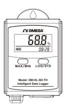
**Start Logging -** When the Logger is on and on stand-by(LCD does not have "LOG" logo display), press "LOG/STD" for 3 seconds, LCD display time, loosen "LOG/STD" button when the LCD display "3.0", now the logger start logging and storing data(LCD has "LOG" logo display).
