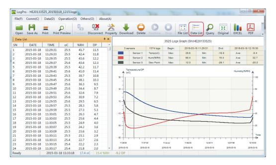
The data pane lists the data samples collected by the logging device. The column width of each column is adjustable by using the left mouse button and dragging the column the desired width.
