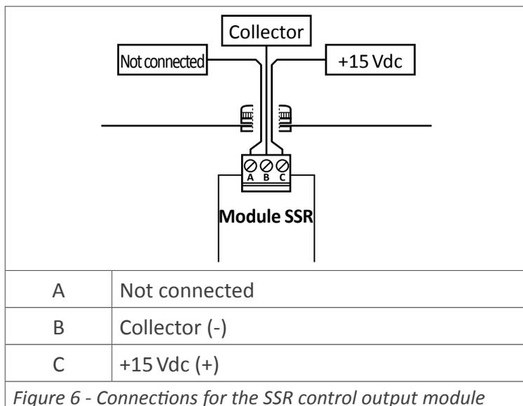
Figure 6 - Connections for the SSR control output module
