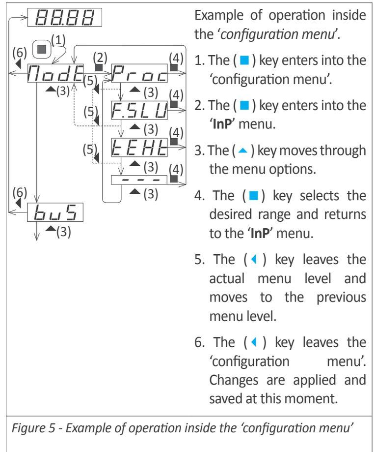
Figure 5 - Example of operation inside the 'configuration menu'
