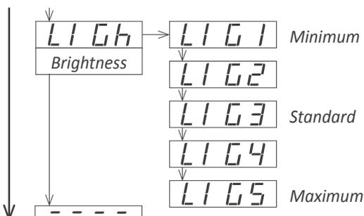
At the 'Brightness' ('LIGh') menu select the intensity level for the display. Use this function to adapt the brightness to match other instruments in the vicinity or to the darkness or clarity of your environment.
