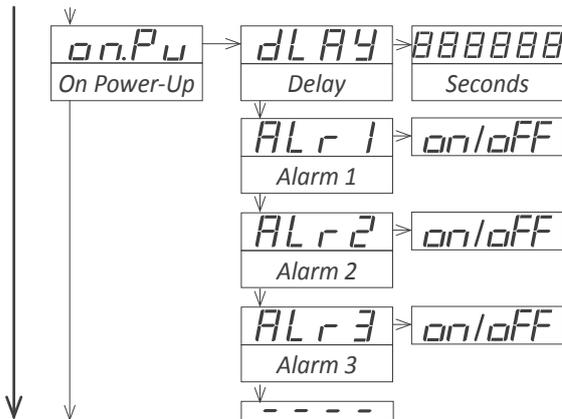
The **'On Power Up' ('on.Pu)'** menu assigns functions to be applied when the instrument starts after a power loss. For more information see section 1.18.12.
