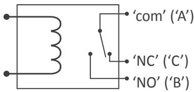
Figure 11 - Module 'R1' and internal schematic
