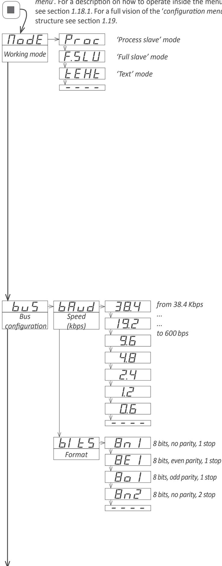
To configure the initial set up of the instrument, select the working mode and configure the bus parameters.
