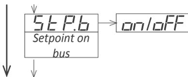
Available in 'Process slave' mode only. Enables access to the alarm setpoint registers through the bus. For more information see section 1.18.13.
