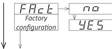
At the 'Factory configuration' ('FAcT') menu select 'yes' to activate the default factory configuration. See section 1.7 for a list of default parameters.
