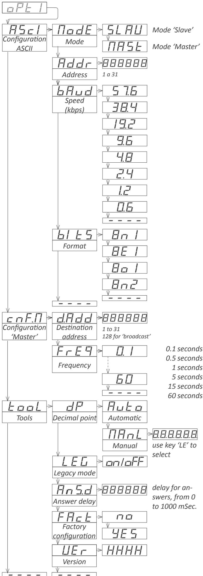
At the 'Configuration ASCII' ('AScl') menu, configure the 'Mode' ('ModE') parameter to select the 'slave' or the 'master' mode, at the 'Address' ('Addr') parameter configure the local port address between '1' and '31', at the 'Speed' ('bAud') parameter select the bus speed (in Kbps) and at the 'Format' ('bltS') parameter select the data format.
