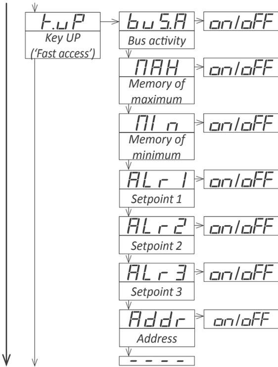
At the **'Key UP ('fast access') ('K.uP)'** menu configure which functions and parameters will be accessible through the 'fast access' menu. Select **'on'** to activate each function. For more information see section 1.18.10.
