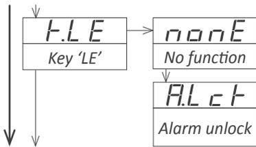
The 'LE' (◀) key at the front of the instrument can be configured to activate several functions. Only one function can be assigned to the 'LE' (◀) key. Eligible functions are the alarm unlock function (see section 1.18.7).
