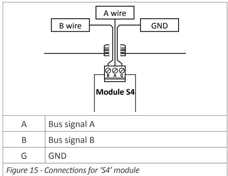
Figure 15 - Connections for 'S4' module
