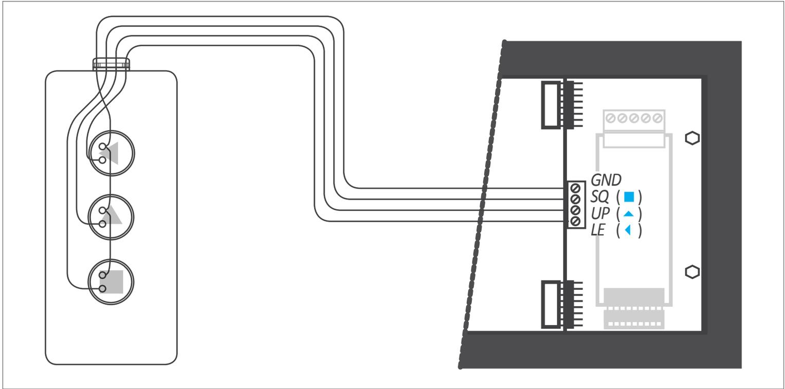
Figure 1 - Connections from RKB to the internal 4 pole terminal
