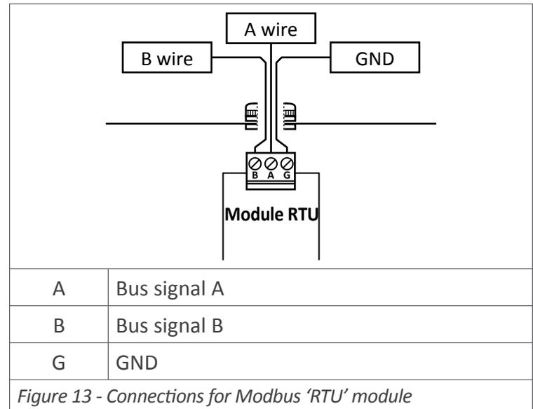
Figure 13 - Connections for Modbus 'RTU' module
