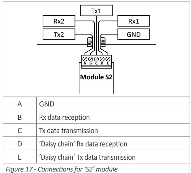
Figure 17 - Connections for 'S2' module
