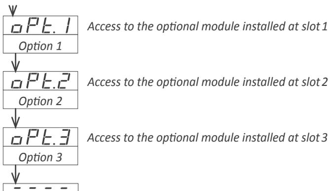
The output and control options are optional modules that can be installed at the instrument. Formats LDB-24 and LDB-44 have 2 free slots for output and control options, while formats LDB-26 and LDB-46 have 3 free slots (see section 1.8).
