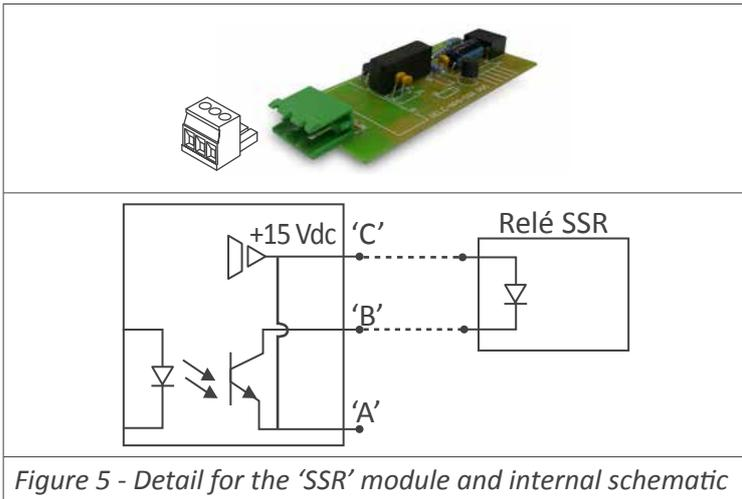
Figure 5 - Detail for the 'SSR' module and internal schematic
