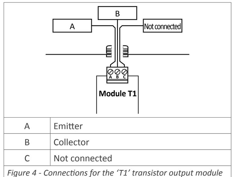
Figure 4 - Connections for the 'T1' transistor output module
