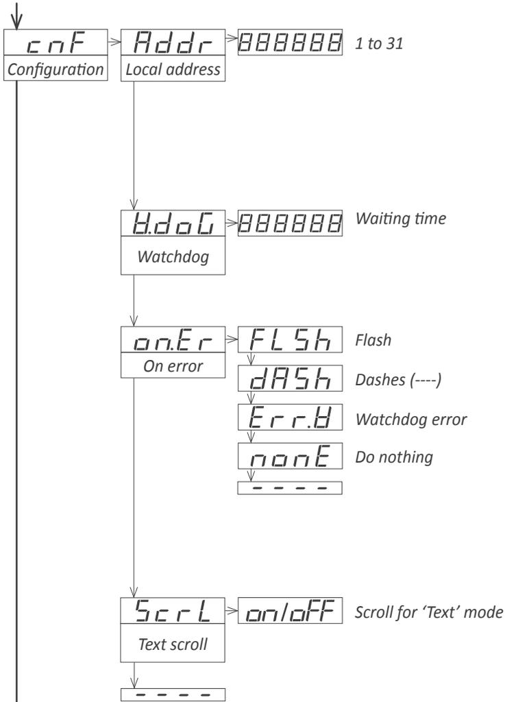
At the '**Configuration**' ('cnF') menu, configure the parameters associated to the instrument function, such as the local address, the 'watchdog' time and error behavior and the scroll in 'Text' mode.
