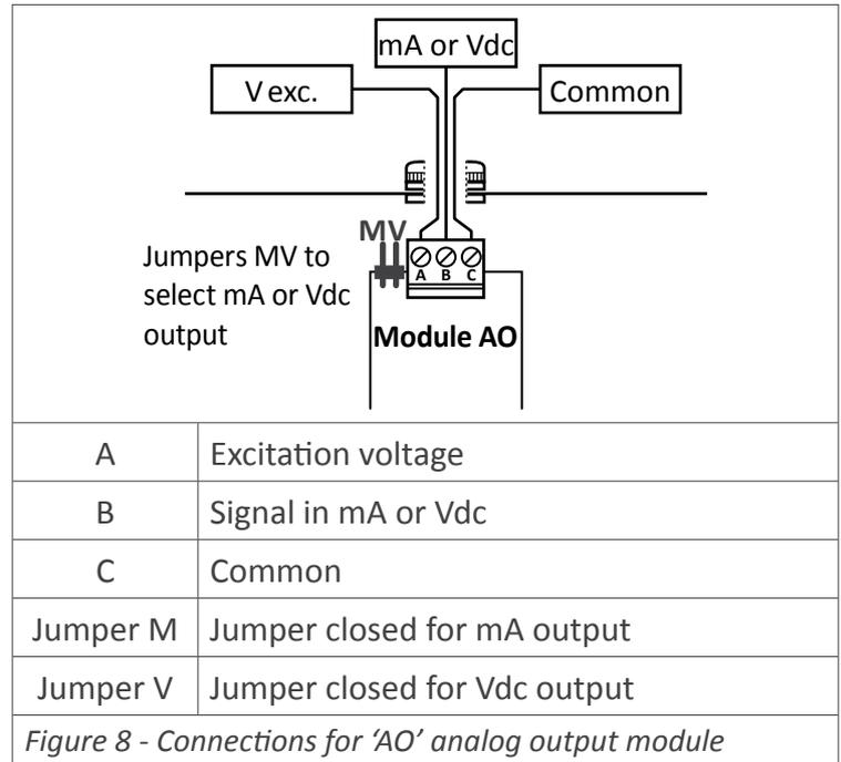
Figure 8 - Connections for 'AO' analog output module
