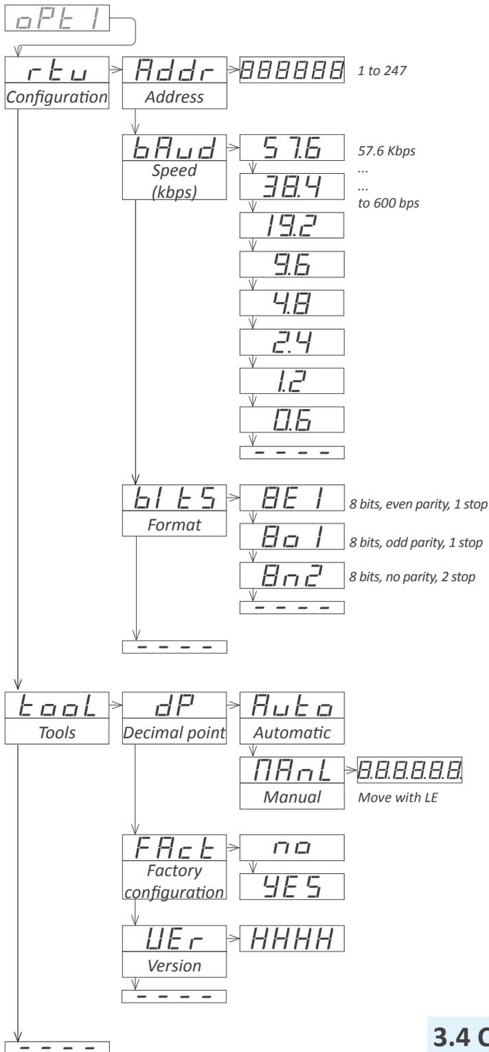
At the 'Configuration' ('rtu') menu, configure the 'Address' ('Addr') parameter with the address value between '1' and '247', at the 'Speed' ('bAud') parameter select the bus speed (in Kbps) and at the 'Format' ('bltS') parameters select the data format.
