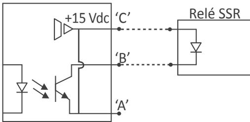
Figure 15 - Module 'SSR' and internal schematic
