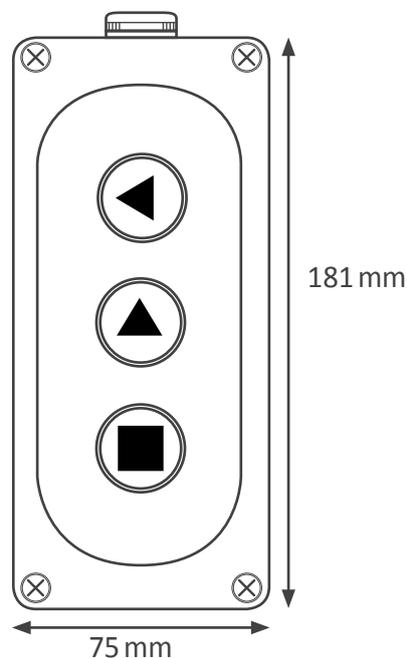
Connect the wire to the 4 pole terminal located close to the input signal module. Connect 4 wires for keys 'SQ' (■), 'UP' (▲), 'LE' (◀) and common. Pass the wires through the cable gland identified as 'remote keypad' (see Figure 2) and connect the other end to the internal RKB push buttons.
