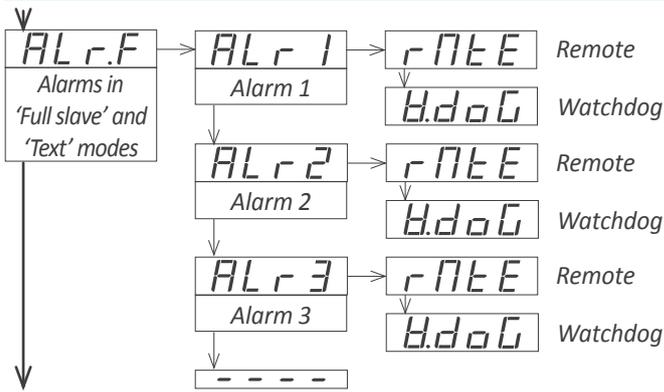
Menu available only in 'Full slave' and 'Text' modes. Alarms are remotely controlled from the bus.
