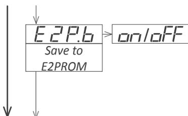
Enables to write to internal E2PROM setpoint values modified from the bus (see section 1.18.14).
