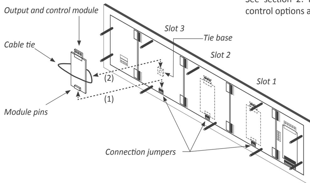
To install an output and control module
