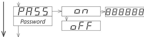
The password function blocks access to the configuration menu. The 'fast access' menu is not affected by the password function. This means that the configuration menu can be password blocked, while some configured functions or parameters can still be accessible to the operator through the 'fast access' menu.
