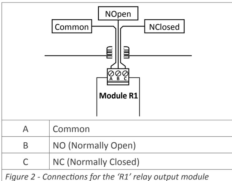
Figure 2 - Connections for the 'R1' relay output module
