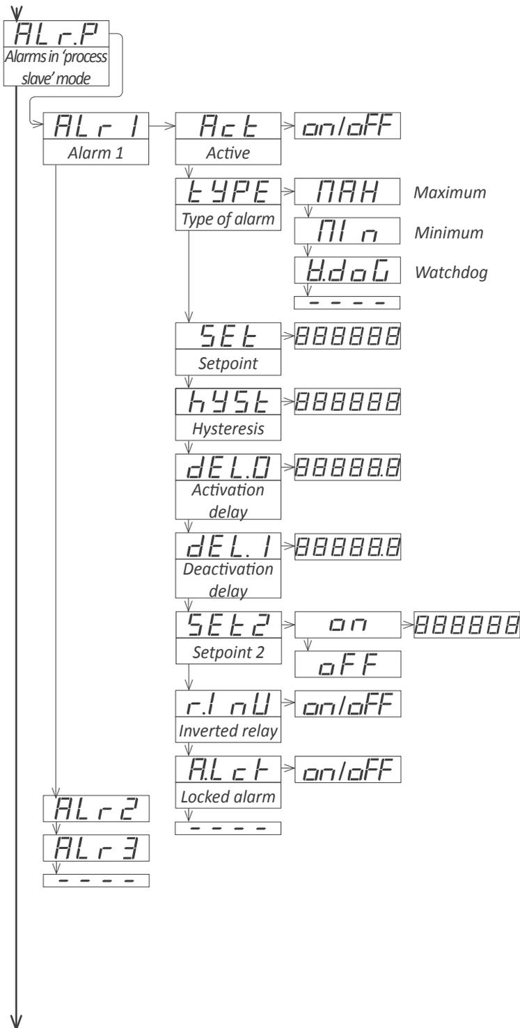
Menu available only in 'Process slave' mode. In 'process slave' mode, alarms are locally controlled from the instrument. Locally configure the alarm parameters for each alarm. For more information see section 1.18.7. At the alarm menu ('ALr1', 'ALr2' or 'ALr3') configure the following parameters:
