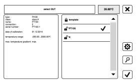
You can use the Licon to switch into expert mode for administering and configuring the test specimens.
