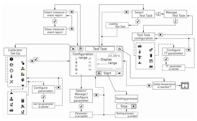
The operating concept of the TCL-3M165E2 is based on pre-installed and self-defined test tasks for recurring testing processes.
