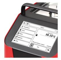
The windows "Calibrator Set Up" and "Select measurement report" are opened with the icons \* and . The window "Select Test Task" is opened from the parameter field with the name of the test task.
