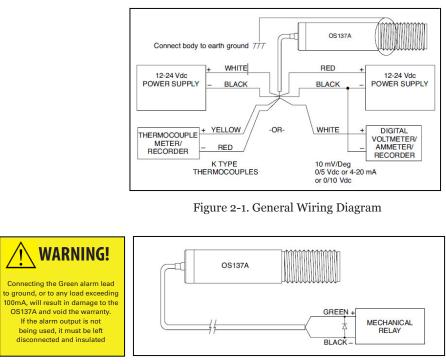
Figure 2-2. Alarm Output Wiring Diagram
