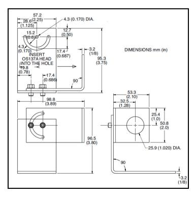
Figure 3-3. Mounting Bracket, OS137-MB
