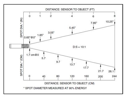
Figure 3-1. Optical Field of View
