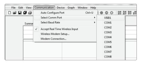
The USB interface can be configured to work with most Omega Data loggers by selecting the proper baud rate from the Select Baud Rate option under the Communications menu. The baud rate used by the logger is listed on its label. For example the OM-CP-Temp101A communicates at 115,200 baud, so 115,200 must be selected.
