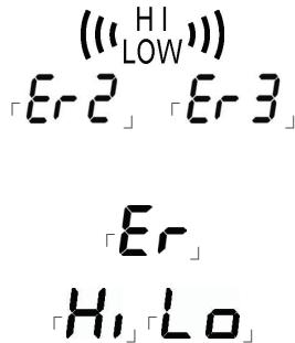
'Hi' or 'Lo' is displayed when the temperature being measured is outside of the settings of HAL and LAL.
