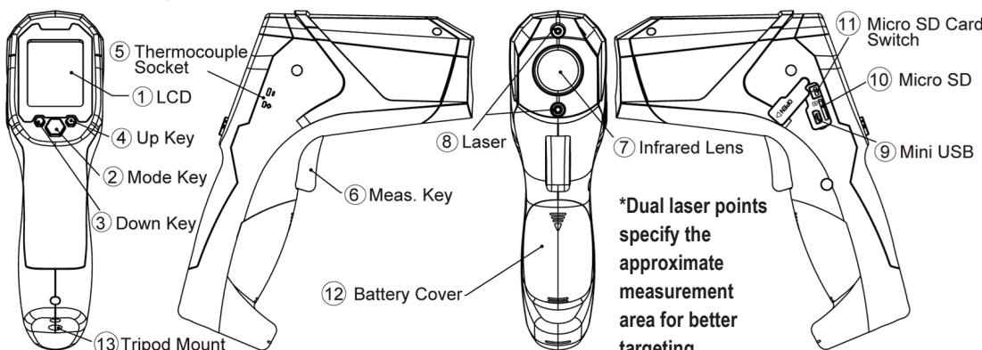
Simply aim the thermometer at the measure target with Lens (⑦) and press Meas. key (⑥) to display the surface temperature. The Distance:Spot is 60:1. Please make sure the target area is within the field of view.
