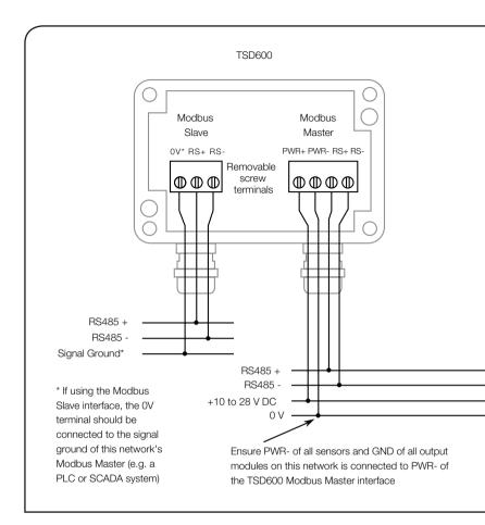
The TSD600 has removable screw terminal blocks for the Modbus Slave and Modbus Master interfaces.
