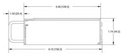
Figure 9. Enclosure dimensions – side
