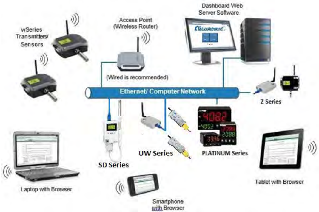
Figure 1.1 Dashboard System on the Ethernet Network
