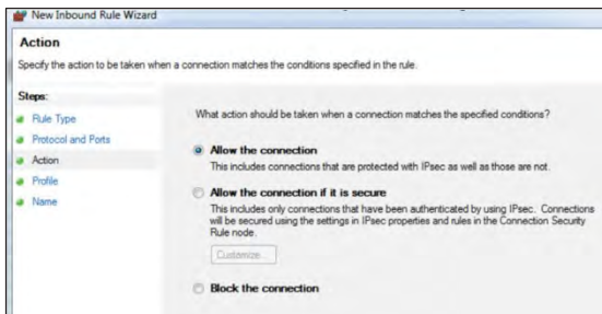
Figure J.9 Windows Firewall - Action
