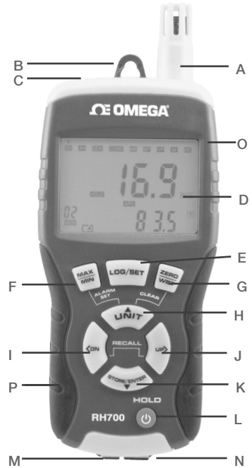
Fig. 1. The controls and physical structures of the RH700
