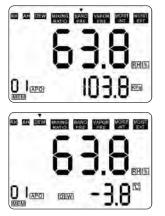
As the figure on the left shows, moving the  $\mathbf{\nabla}$  pointer four positions to the right (by pressing the **UP>** button four times) switches the meter to operate in Ambient pressure mode.
