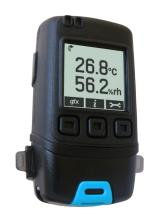
The OM-EL-GFX-2-PLUS standalone USB data logger measures and stores up to 252,928 temperature and humidity readings over a -30 to  $+80^{\circ}$ C (-22 to  $176^{\circ}$ F) and 0 to 100%RH range at a resolution of  $0.1^{\circ}$ C ( $0.1^{\circ}$ F) and 0.1%RH.
