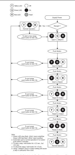
Figure 1: DRI-U-AC Calibration Flow Chart
