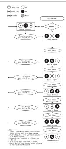
Figure 1: DRI-U-DC Calibration Flow Chart
