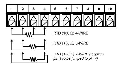
Figure 5 – RTD Wiring Diagram
