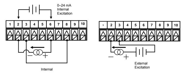
Figure 6 – Process Current Wiring Hookup with Internal and External Excitation
