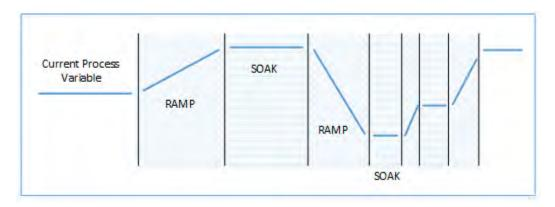
Figure 15. Ramp & Soak Current Process Variable.
