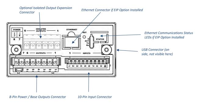
Figure 2 – CN8Pt, CN8DPt and CN8EPt Models: Back Panel Connections (With Isolated Output Expansion Board)
