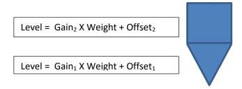
A 10-point linearization table is provided, allowing for piecewise linearization of complex profiles. This feature is often used to transform weight values into volume or to transform primary measurements into derived measurements such as rate of change in temperature to air flow.
