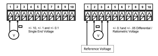
Figure 7 – Process Voltage Wiring Hookup with optional Ratiometric Voltage connection.
