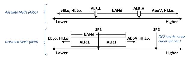
Figure 10 – Alarm Range Option Diagram
