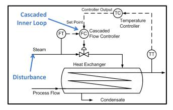
Figure 12 Generic Cascade Control Diagram
