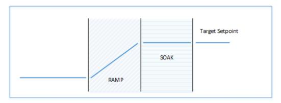
Figure 14. Ramp & Soak Process Variable Period of Time.
