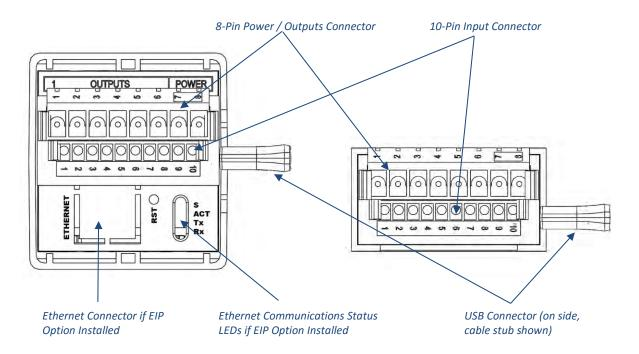
Figure 3 – CN16Pt and CN32Pt Models: Back Panel Connections
